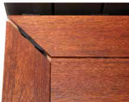
Creating a Mitre Butt-End Joint
